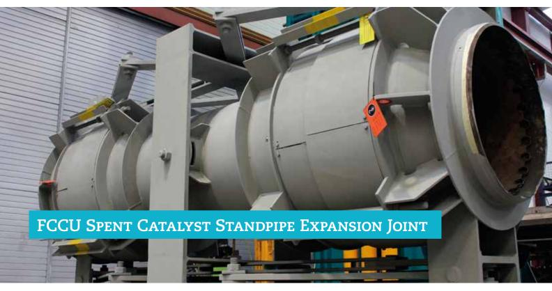
A high-tech FCCU Spent Catalyst Standpipe Expansion Joint has been manufactured, designed, tested and delivered for a refinery in South America.
